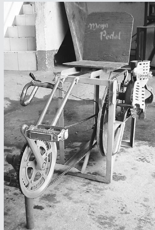
Figure 2.6 Maya Pedal's Bicidesgranadora (Corn Sheller)
