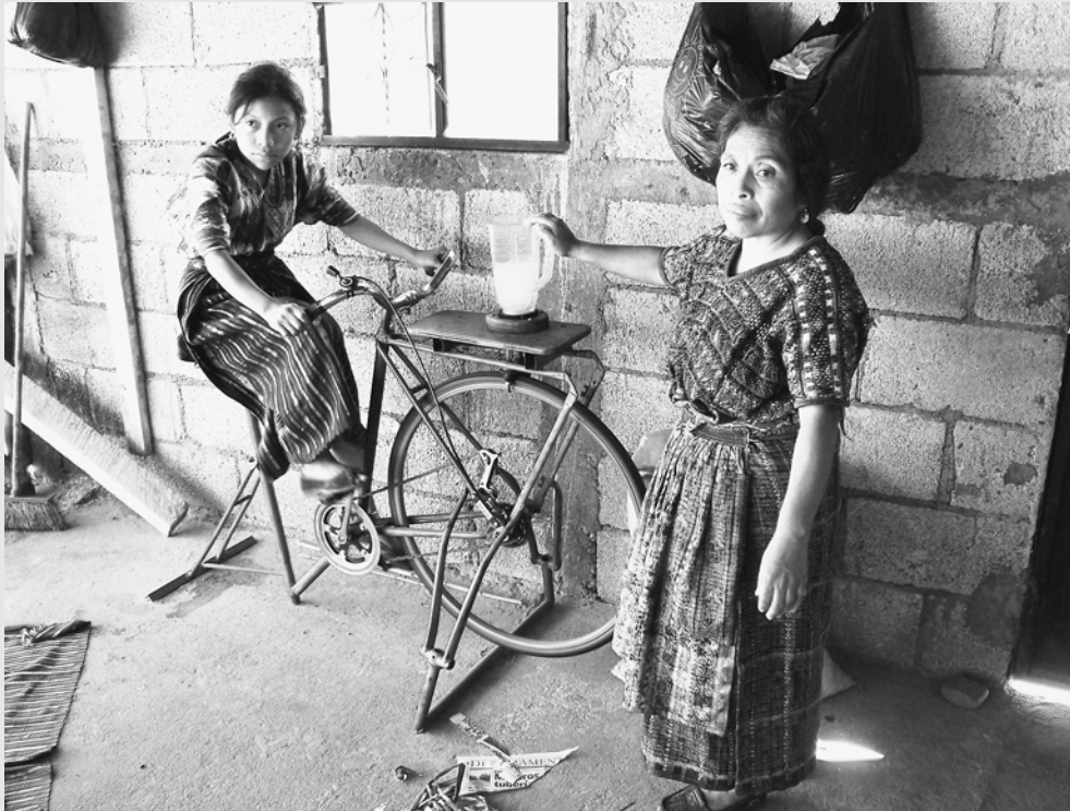
Figure 2.7 Maya Pedal’s Bicilicuada (Blender)
