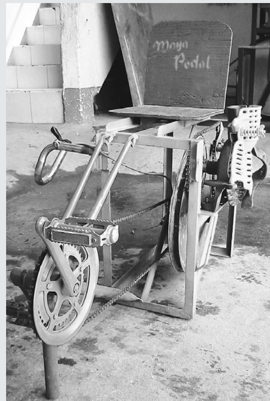
Figure 2.6 Maya Pedal's Bicidesgranadora (Corn Sheller)
