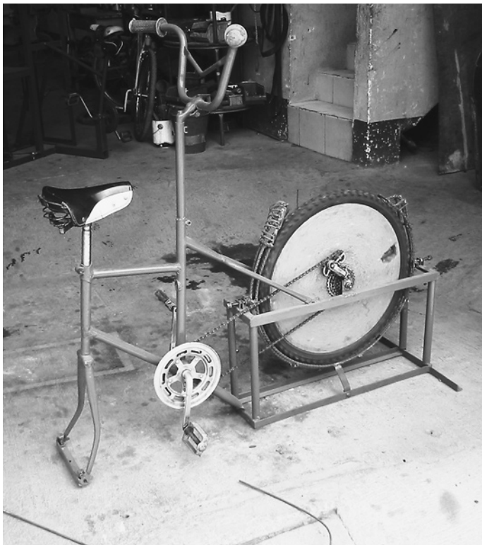
Figure 2.21 Maya Pedal's Bicimacadamia (Macadamia Nut Sheller)
